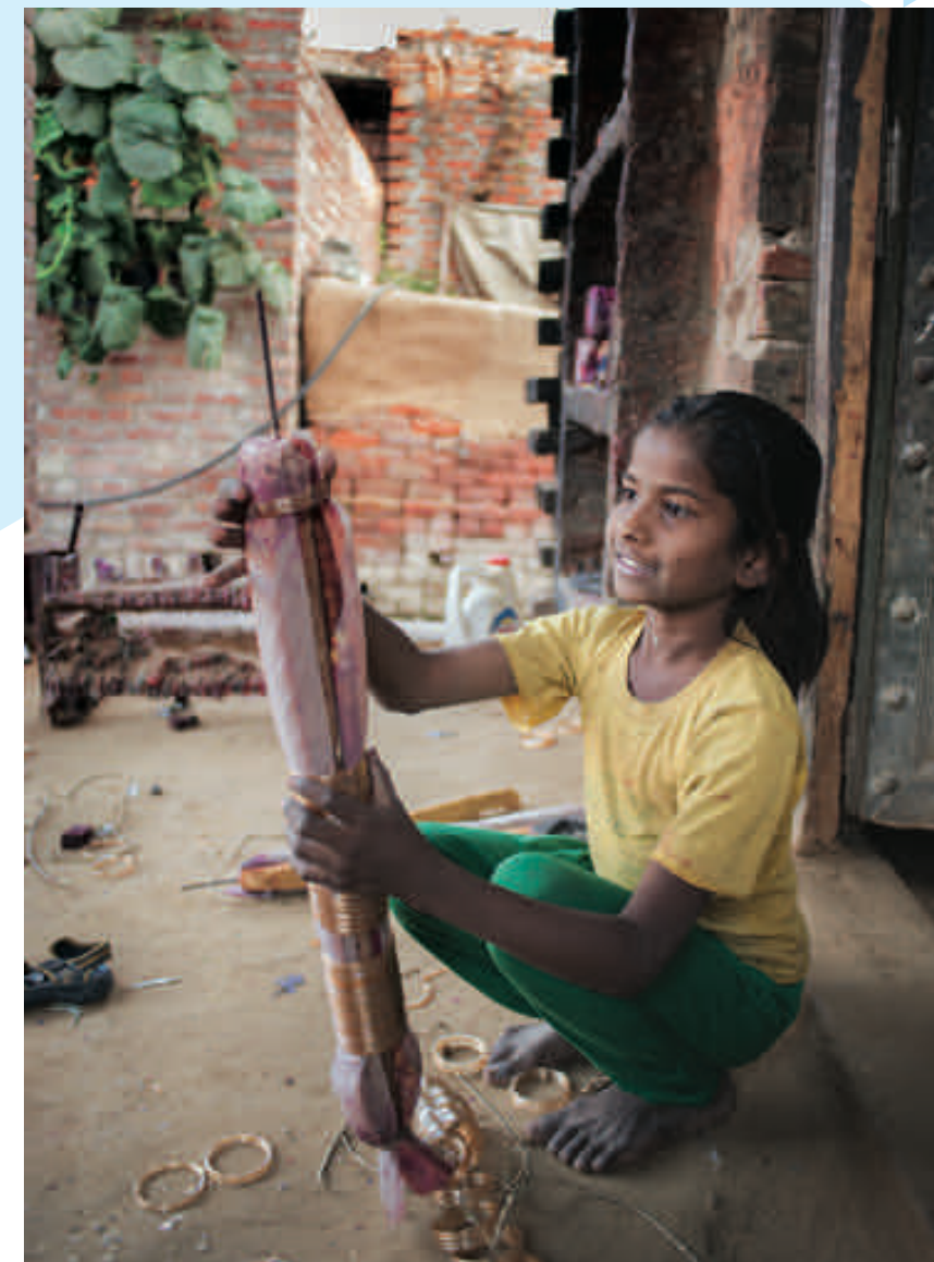
▲ A girl loads bangles onto a rolling pin before embellishing them with glittering coats
