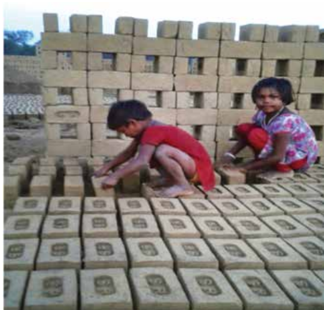
Rotating bricks for drying ( Thalana )
